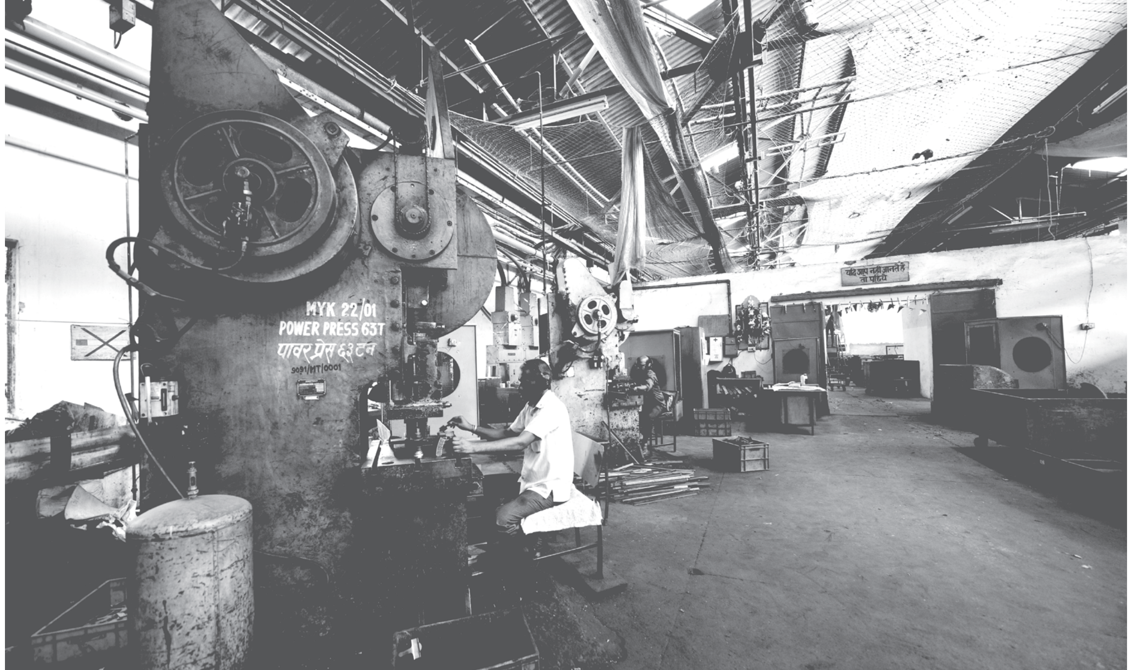
Existing Press Shop (Old) for production of sheet metal parts for T/c, MTC, WC Rollators and Orthotic lower components
