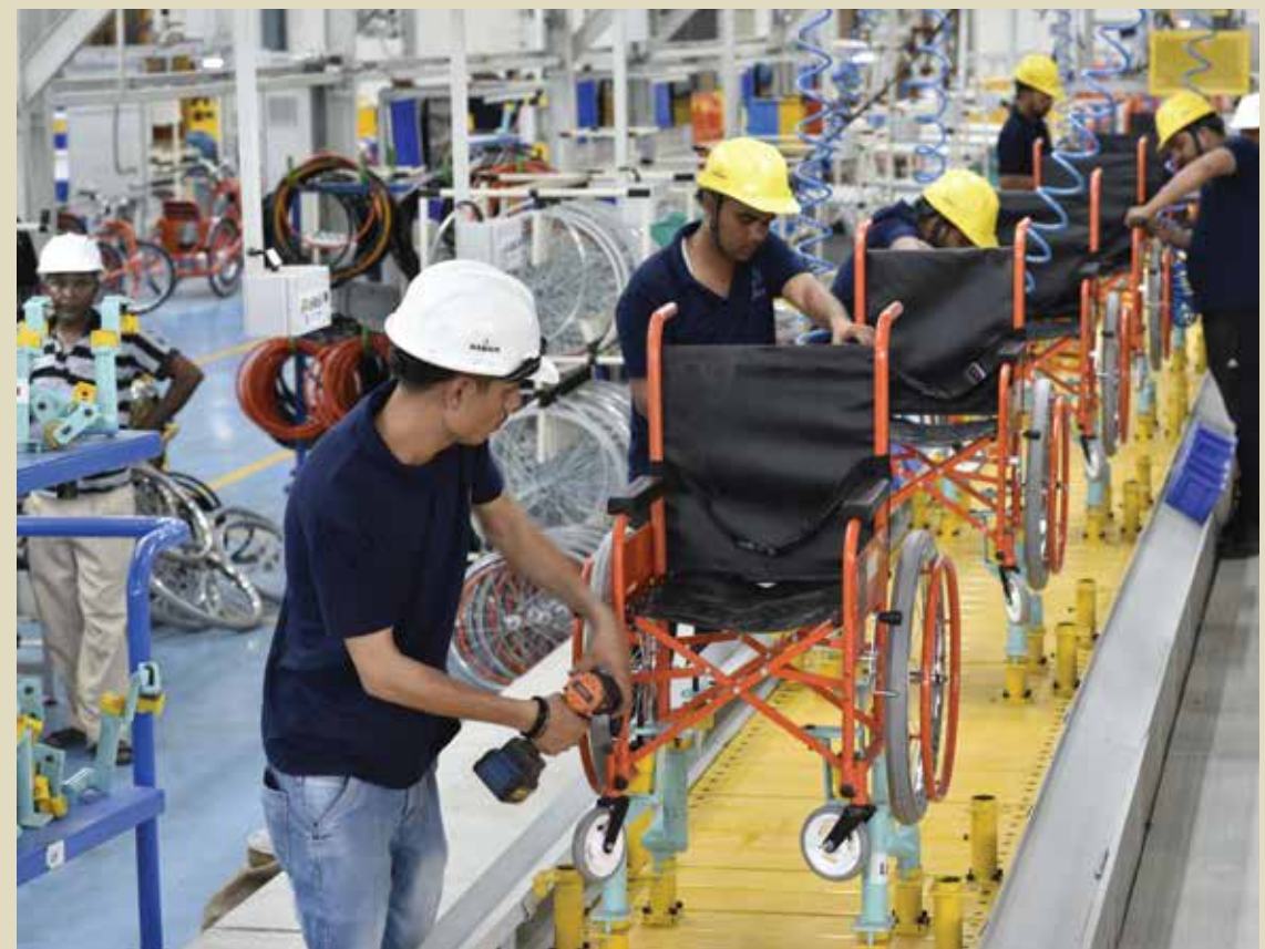
Wheelchair frames being set as per specifications
