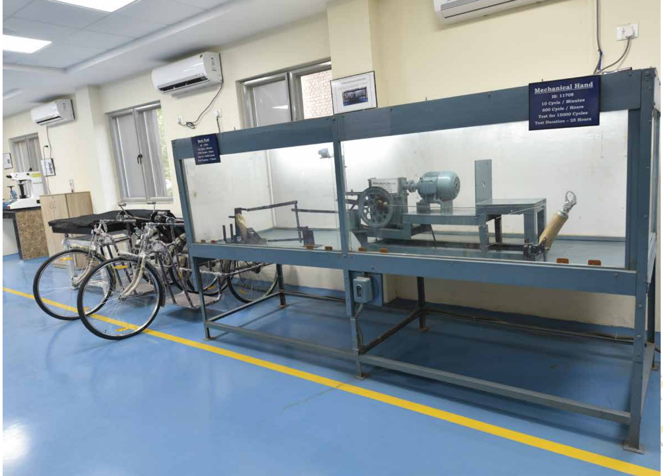
Quality test of Mechanical Hand through Cyclic Test procedure for 15000 cycle of as per IS : 11708
