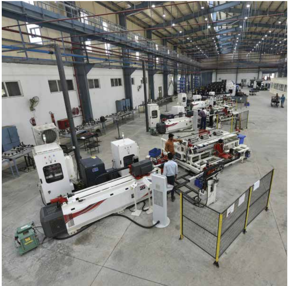
Work Centre - 2 (New Tube and sheet preparation shop) 3 axis & 5 axis bending machines, laser tube and sheet cutting machine. (WC/MTC/TC/Rollators)
