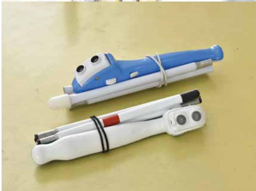
Sugamya Cane: Inhouse developed, designed and manufactured electronic cane for visually impaired
